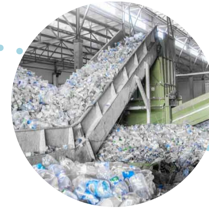
In the sorting plant plastic waste is classified by plastic type
