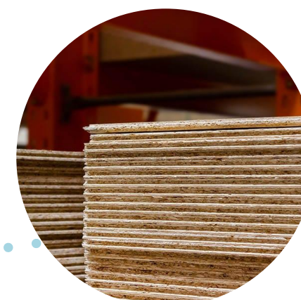
The majority of the shredded material will be transformed into recycled wood planks of lower quality chipboard. When material does not meet quality requirements it is burned
