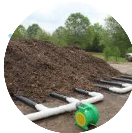
At composting facilities a biologic process treatment with oxygen takes place from which compost is obtained
