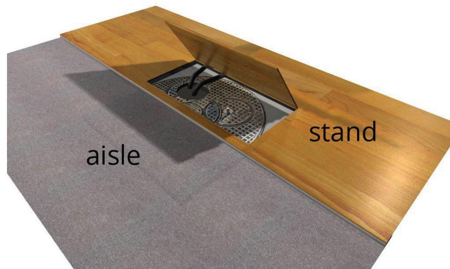
Whenever a service chest is half covered by a division wall or is at the limit of the stand, the area around the chest must remain accessible.
