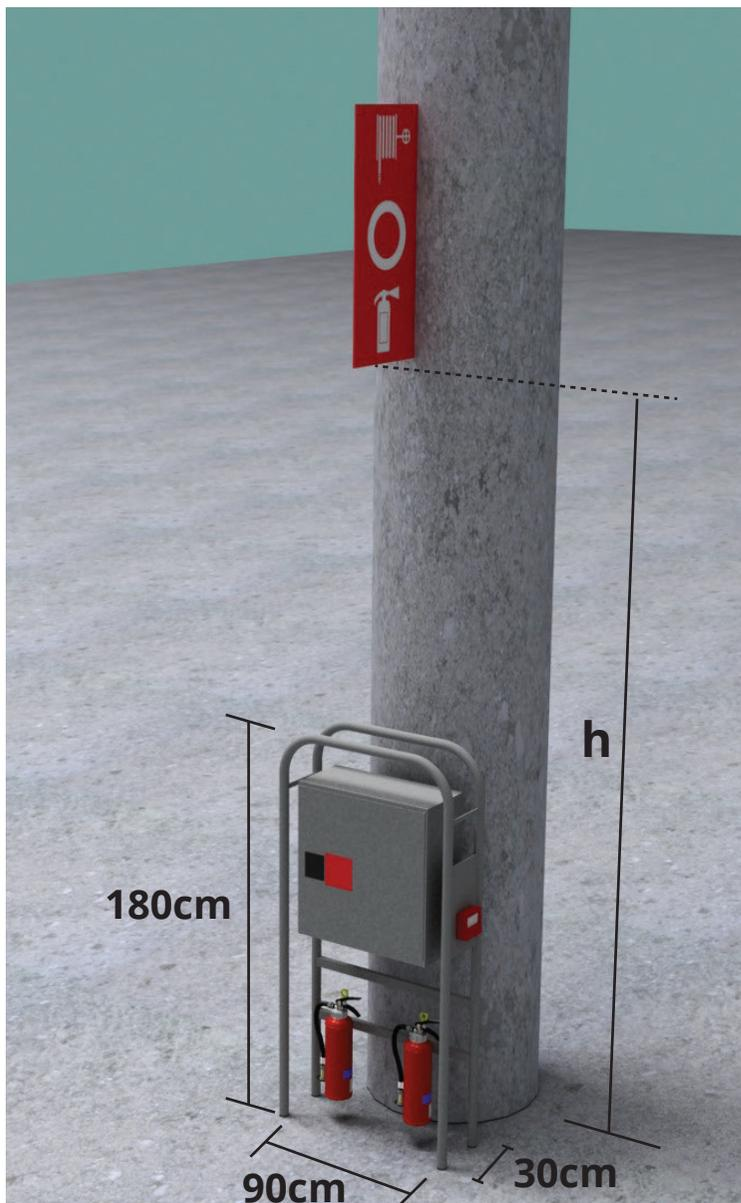
Note that the fire extinguisher equipment can only be cladded if all the equipment remains accessible at all times.
