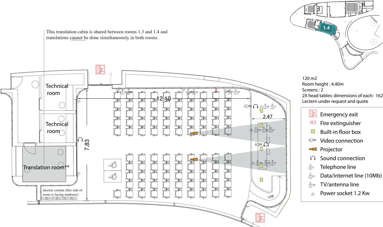
AV installed in the room: PA System, Screen frontal 600x340cm automatic, 2 independent projections 300x225 (4:3) or 300 X 168 (16:9), 2 projectors 6000 lumens HD projector, HDMI input, 4 table /lectern mics, 1 wireless mic (handheld or headset), 2 fixed cameras, translation booth digital, PC laptop, laser presenter. The AV technician is not included. Contact our team for a quote.
