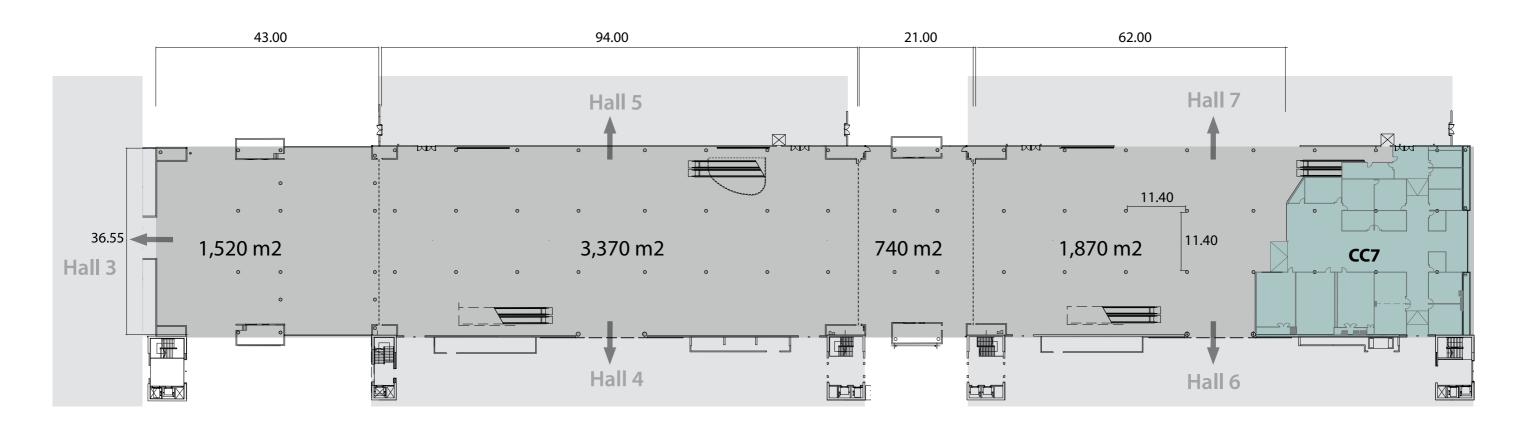
height: 5,20m / max construction height 4m ground resistance 1.000 kg/m2
