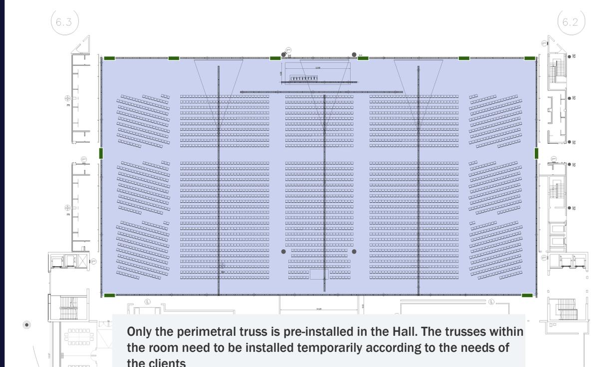
Only the perimetral truss is pre-installed in the Hall. The trusses within the room need to be installed temporarily according to the needs of the clients
